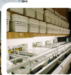
The Outpatient Pharmacy Automation System is an intelligent conveyor system to dispense medication at the Singapore General Hospital
