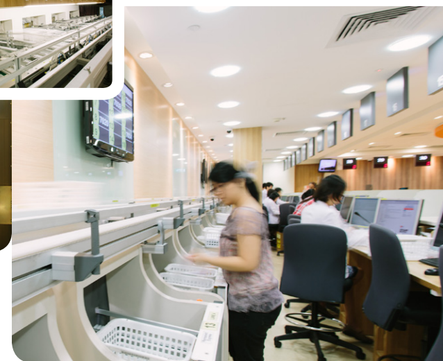
The Outpatient Pharmacy Automation System is an intelligent conveyor system to dispense medication at the Singapore General Hospital
